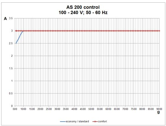
Fig. 11: Load diagram for the sieve clamping units "economy", "standard" and "comfort"
